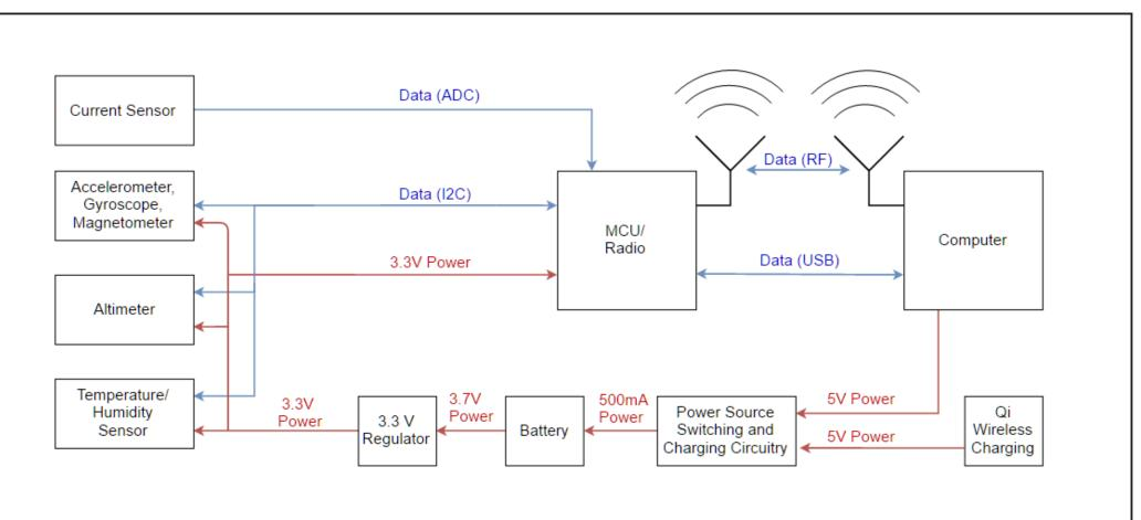
Figure 2: PatSTARS module block diagram
