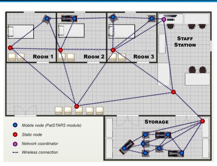
**Figure 3:** Example PatSTARS network configuration
