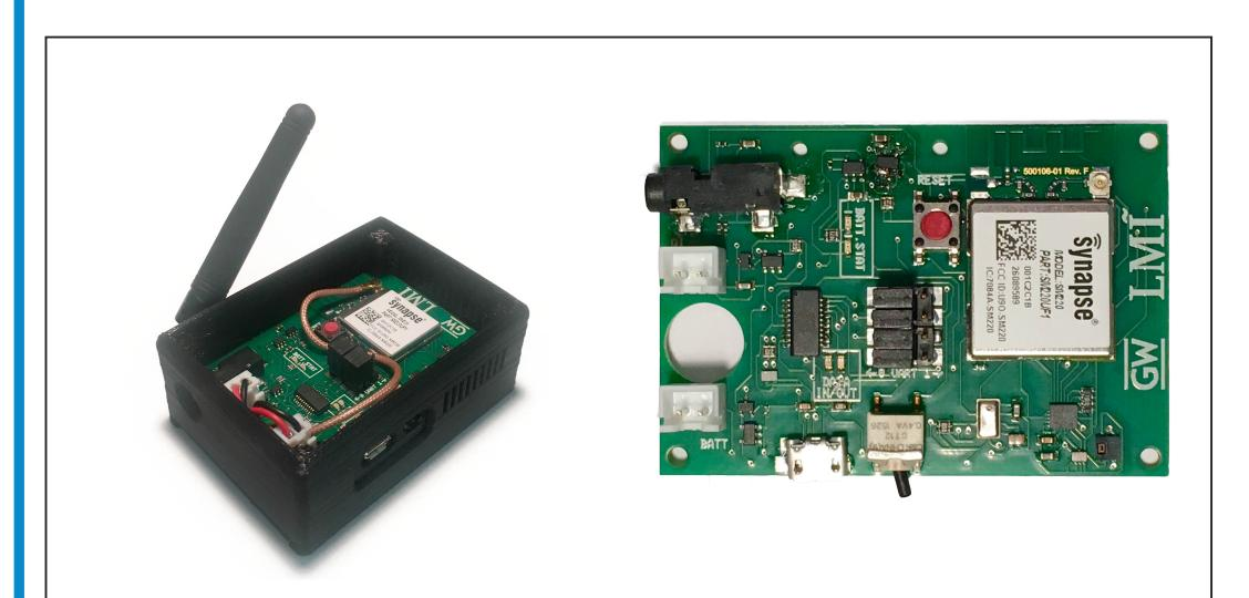
**Figure 1:** PatSTARS module (*left*); internal circuitry (*right*)
