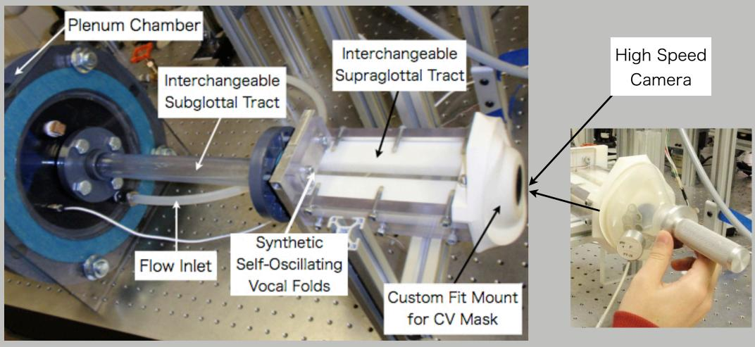
Figure 2.1 - Experimental Setup
