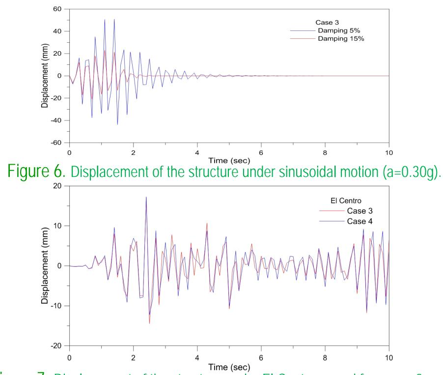
Figure 7. Displacement of the structure under El Centro record for cases 3 and 4 with 5% of damping.
