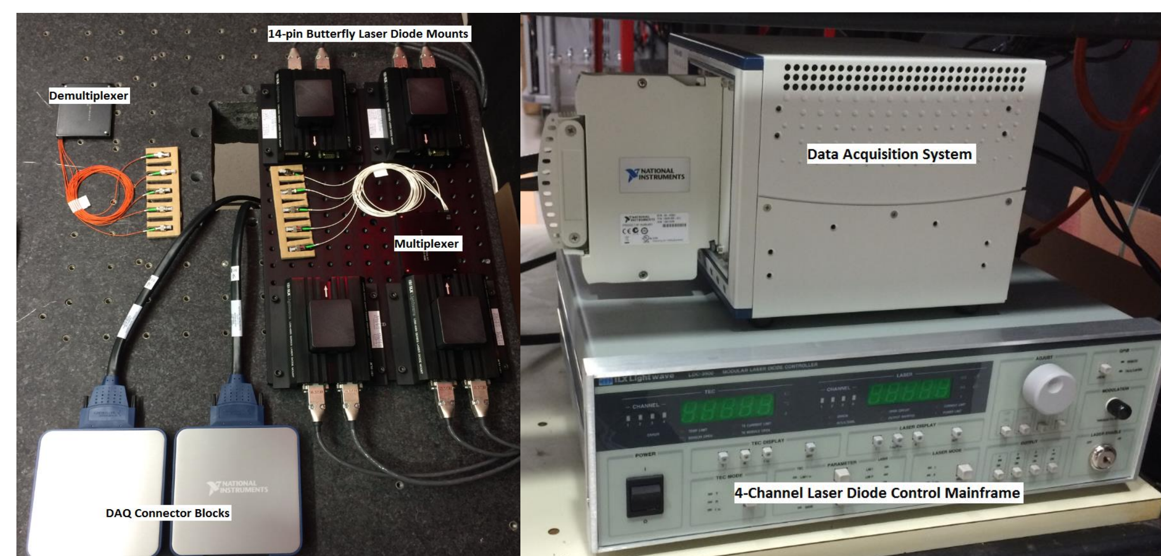
Fig. 6: DFB mounts, Mux/Demux system, DAQ, and laser current/temperature controller
