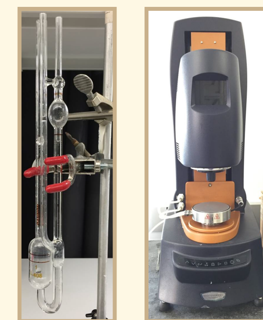
Figure 4: Ubbelohde Viscometer, Rheometer
