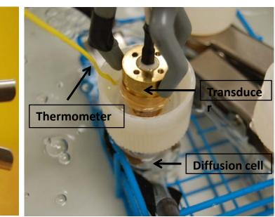
• Ultrasound was applied with intensity of 0.3, 0.5, 0.8, and 1 W/cm<sup>2</sup> at different frequencies of 400 KHz, 600 KHz, 800 KHz, and 1 MHz with application duration of 5 min.
