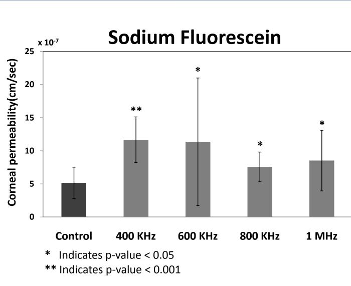
In case of Sodium Fluorescein, ultrasound application for 5 minutes at 1.0 W/cm<sup>2</sup> produced permeability increase of 126% at 400 KHz (n=9), 121% at 600 KHz (n=13), 47% at 800 KHz (n=9), and 65% at 1 MHz (n=12) as compared to sham treated cases (n=9).
